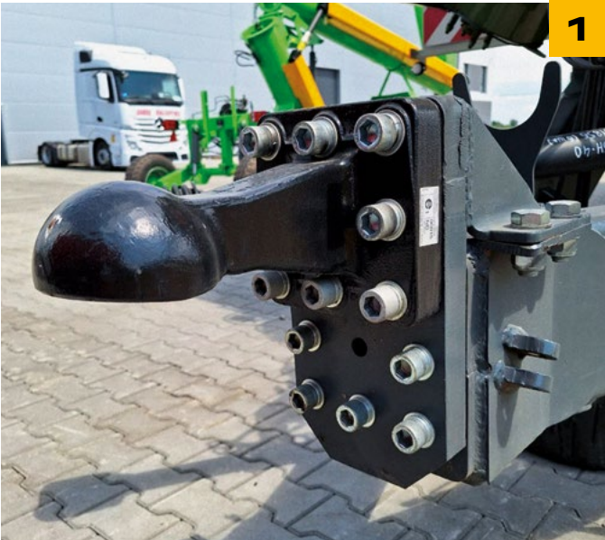
HEIGHT ADJUSTMENT ADAPTER FOR CONNECTION TO ANY TRACTOR
