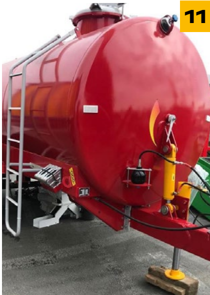
ADJUSTING THE MOUNTING HEIGHT AND BARREL TILT
