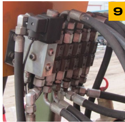
EELECTRICAL UNIT FOR CONNECTING 5 PAIRS OF OUTPUTS
