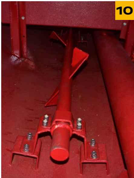
MECHANICAL MIXER WITH HYDRAULIC DRIVE
