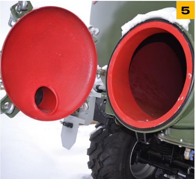
INTERIOR BARREL TREATMENT WITH POLYMER COATING
