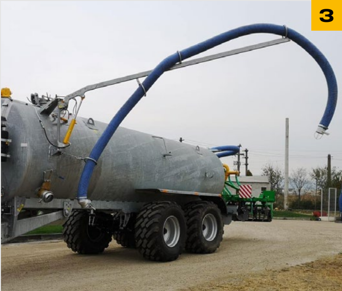
HYDRAULIC MANIPULATOR MATERIAL PUMPING HOSE
