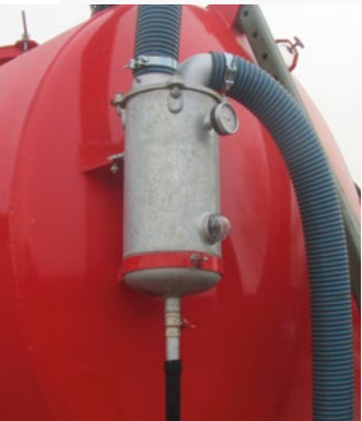
Siphon prevents slurry from entering the pump
