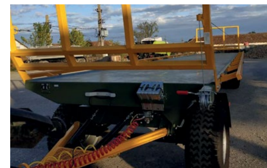
Winch and broadening of platform to 3 m
