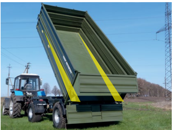
Conical body prevents of hanging green mass and fertilizers
