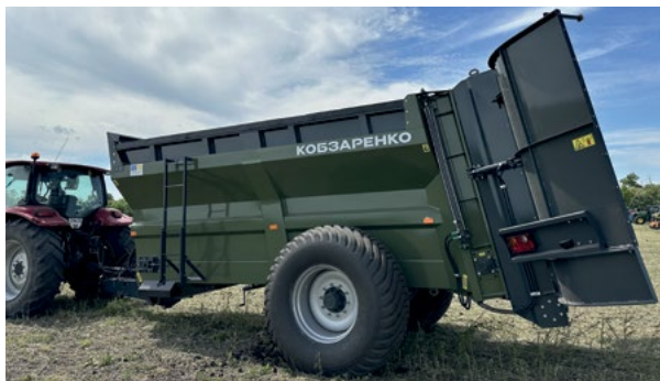
Rear wall opened hydraulically
