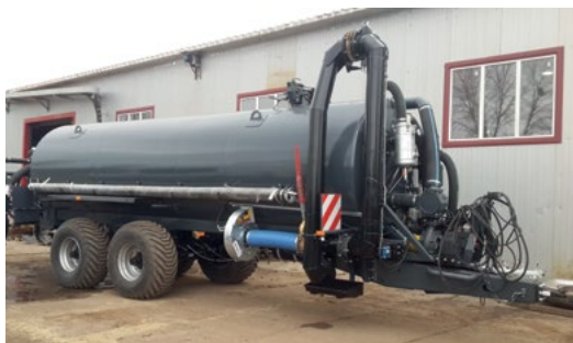
Anti-corrosion coating with polymer paints, hydraulic mixer
