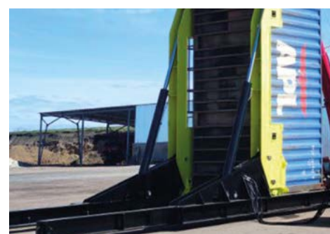
Reinforced hydraulic cylinders for lifting / lowering
