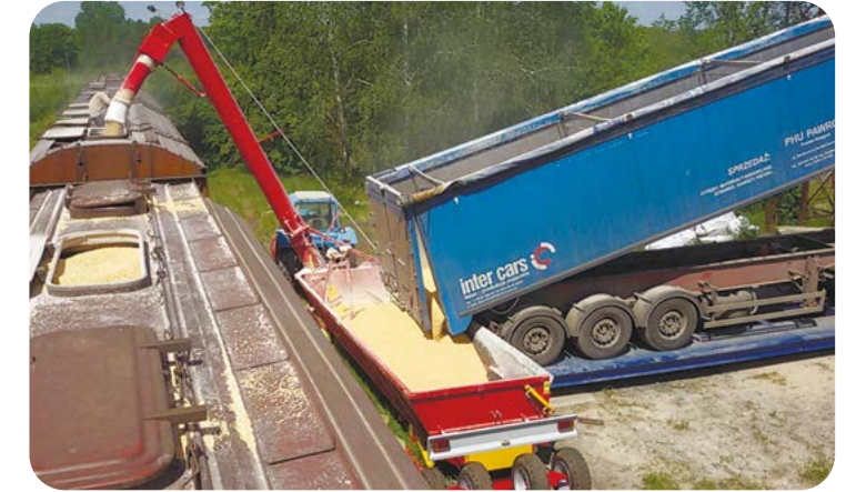
BNP-12 "KOVCHEG" - LOADING HOPPER CARS
