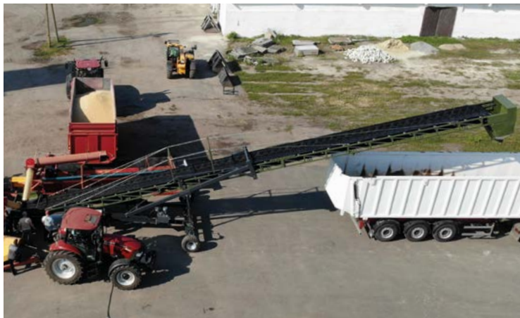
The length of the conveyor is 22 m.
