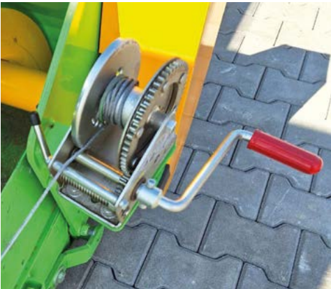
Winch for installing sides
