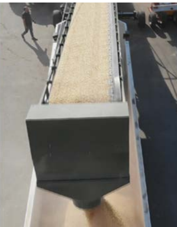
The V-shaped chevron belt 1 250 mm does not damage the seeds
