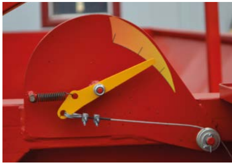
Scale that shows opening of the slide gate
