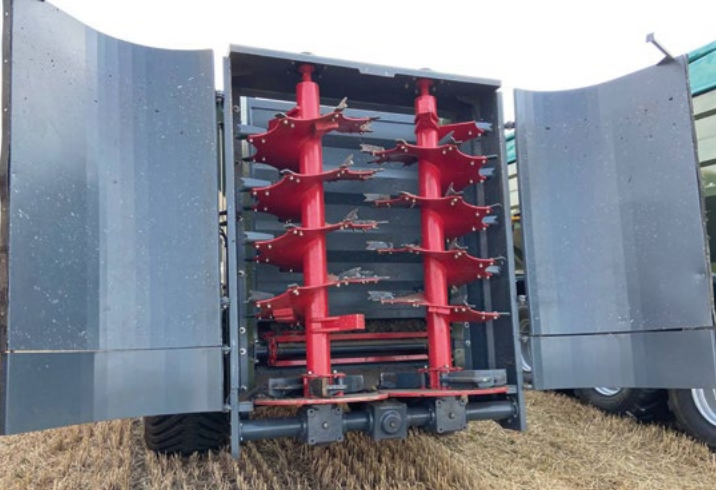
Vertical spreading rollers
