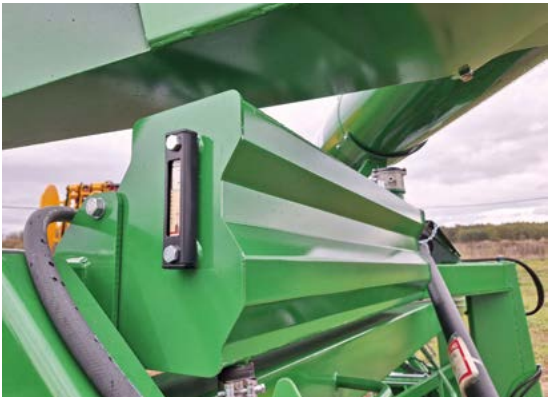
Additional oil tank with thermometer
