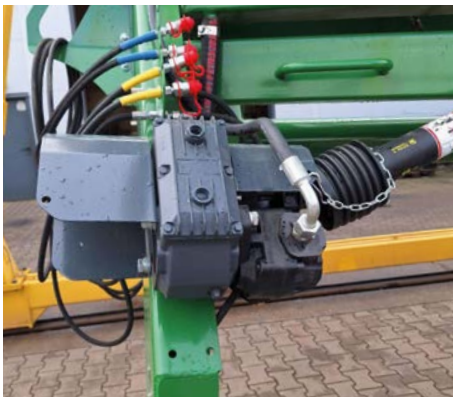
Autonomous oil station on ZRM-180. To increase the flow of oil on the hydraulic motor.
