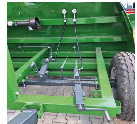
Brake system pressure adjustment for each wheel separately
