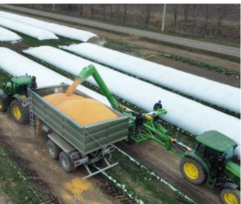
The height of discharge from the sleeves is 4.3 m.
