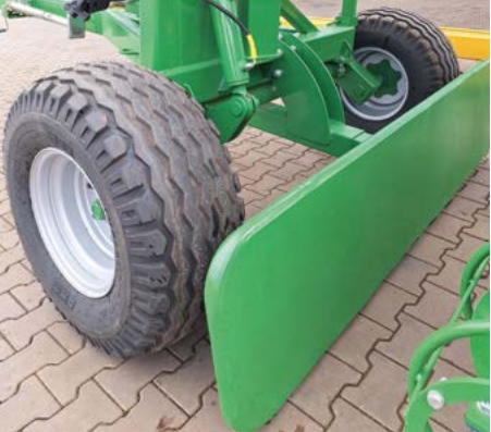
Protective bump what prevent wheels from hitting on bag
