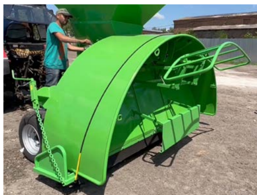
Raising/lowering the frame on which the sleeve lies - with a winch
