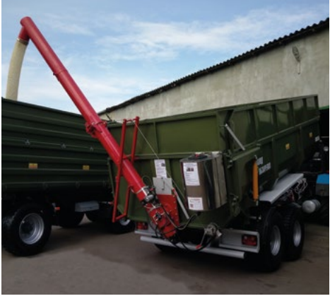
Auger on trailer with rear unloading
