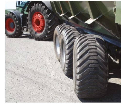
First and last axles are positively steered
