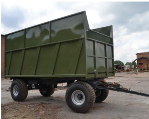
2TSP-14 chip carriers with a body volume of 24 m³
