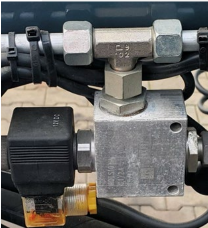
HYDRAULIC VALVE TO BLOCK OPENING OF THE SLIDING GATE AT FIXED PTO
