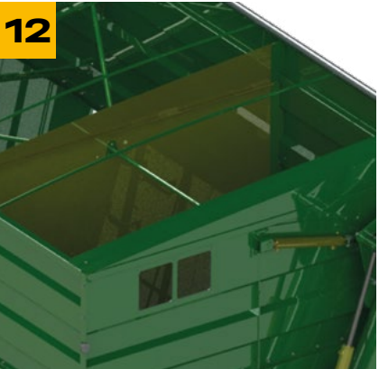
DEVIDING OF THE BUNKER INTO TWO PARTS
