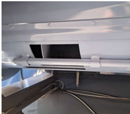
THREE CLEANING FLAPS OF HORIZONTAL AUGER
