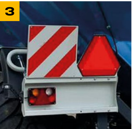
ROAD LIGHTING OF THE TRAILER ACCORDING TO EU STANDARDS
