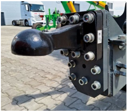
ADAPTER FOR HEIGHT ADJUSTMENT TO HITCH TO ANY TRACTOR
