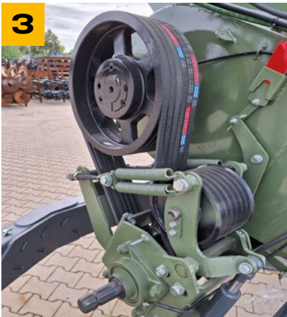
SEPARATE DRIVE WITH ALTERNATE INCLUSION OF AUGERS
