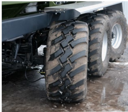
A HYDRAULICALLY STEERING FIRST AND LAST AXLES (PBN-40 AND PBN-50).
