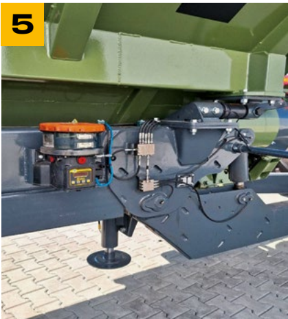
PROGRAMMABLE COMPUTER WITH PRECISE BEARING LUBRICATION INTERVAL
