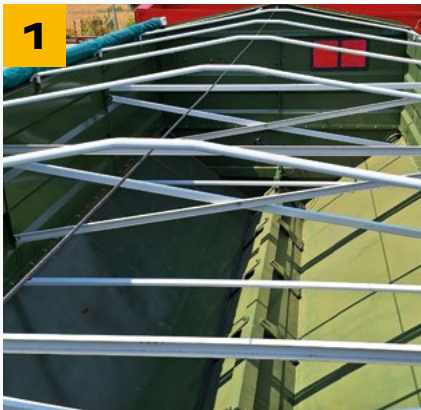
THE SIDES OF THE BODY ARE PULLED TOGETHER BY POWERFUL PROFILE SPACERS
