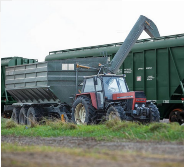
EXTENDED AUGER H-5.5 M FOR LOADING WAGONS
