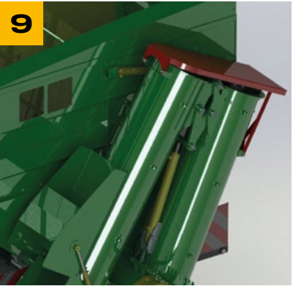
PROTECTIVE COVER OF THE AUGER AGAINST PRECIPITATION
