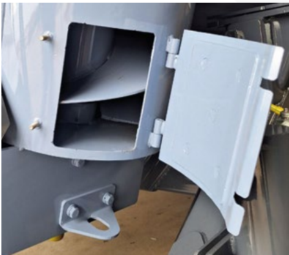
ONE HATCH FOR CLEANING OF VERTICAL AUGER
