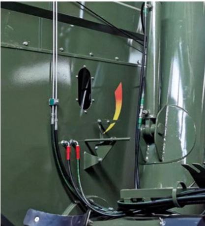
INDICATOR OF SLIDE GATE OPENING
